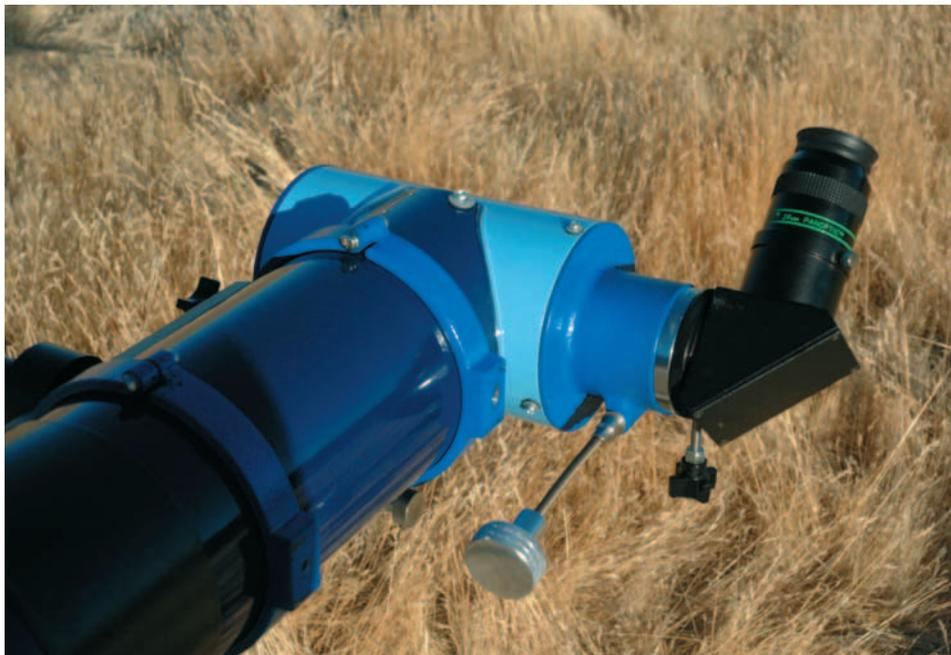
The key to the scope's design is the ability to adjust the tilt of the eyepiece independent of the telescope tube's orientation. This is accomplished by adjusting the angle of the RFT's star diagonal.
